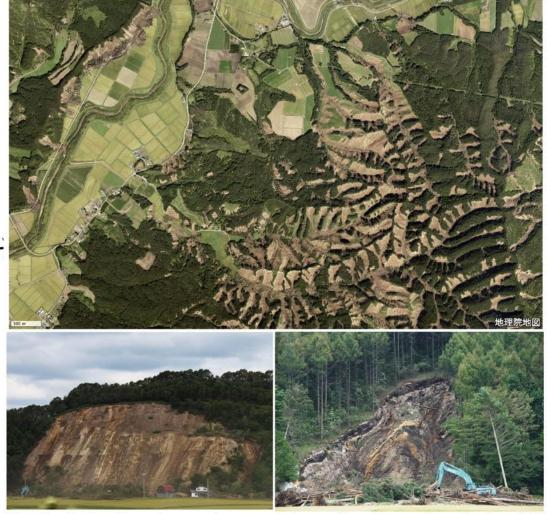
Fig. B Orthophoto image (upper; 5 days after the earthquake by GSI Japan) and photos of typical failured slope (lower).
