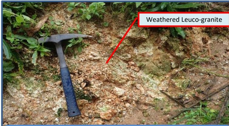
4. Earth material on the slope is mainly composed of weathered leuco-granite (Sandy soil).
