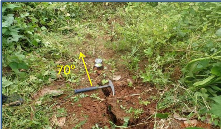
6. Local fault and direction of crack signs. (Generally = 70°)
